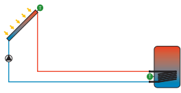
Internal heat exchanger, intelligent pump control
